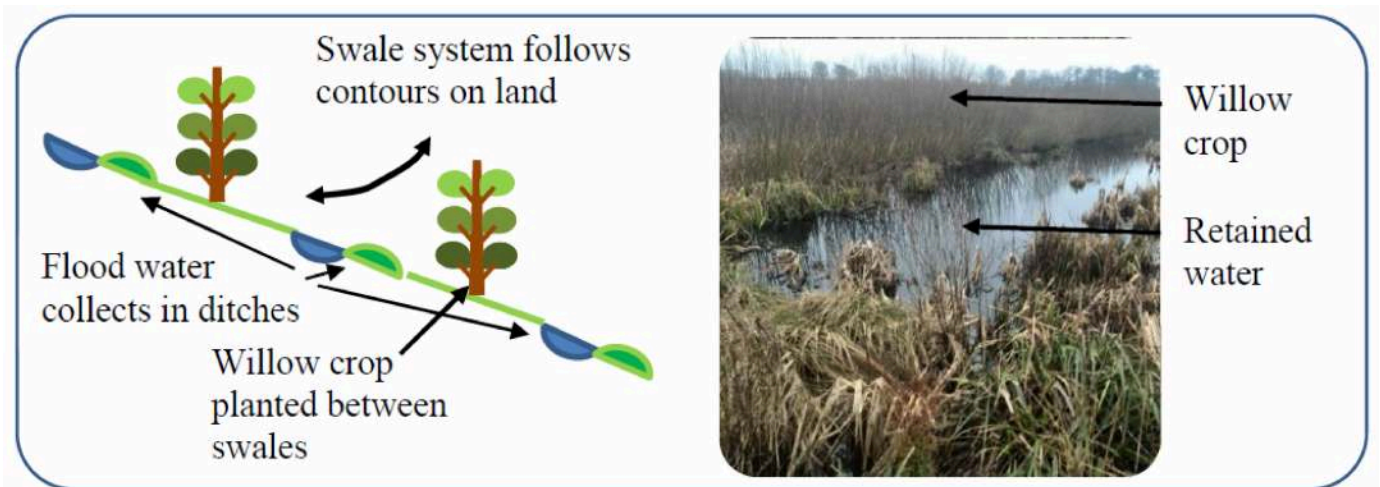
Fig. 4 A simplified arrangement of swales along the field (left), a willow site with swales
